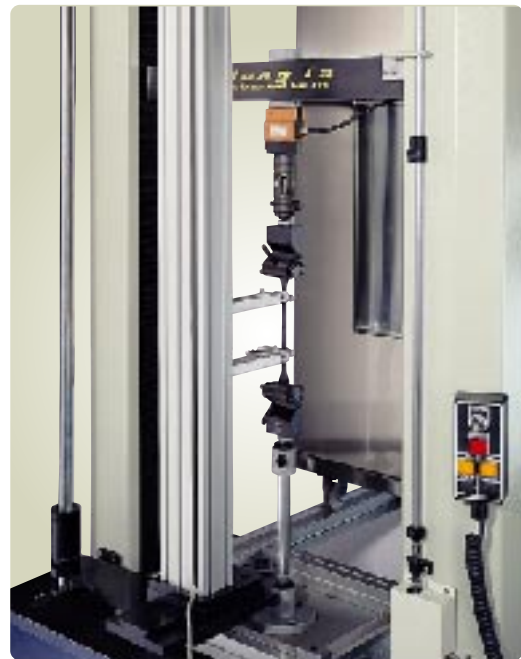
HT-8160 Two extensometer can be selected together with HT-8747 series chambers, but cannot be used at the same time.
