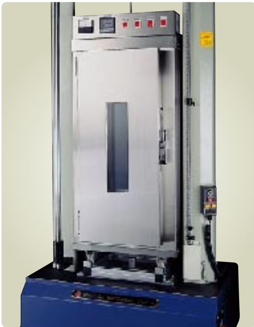
HT-8747 A / B / C Type Thermostat testing chamber HT-2402 / HT-2102 / HT-9102 / HT-8503 For capacities less than 20kN, it is suitable for special (wider ) type 560 mm only
